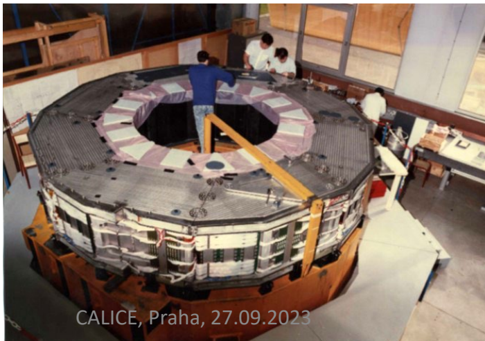
Hadron barrel calorimeter assembly at LAL Orsay
