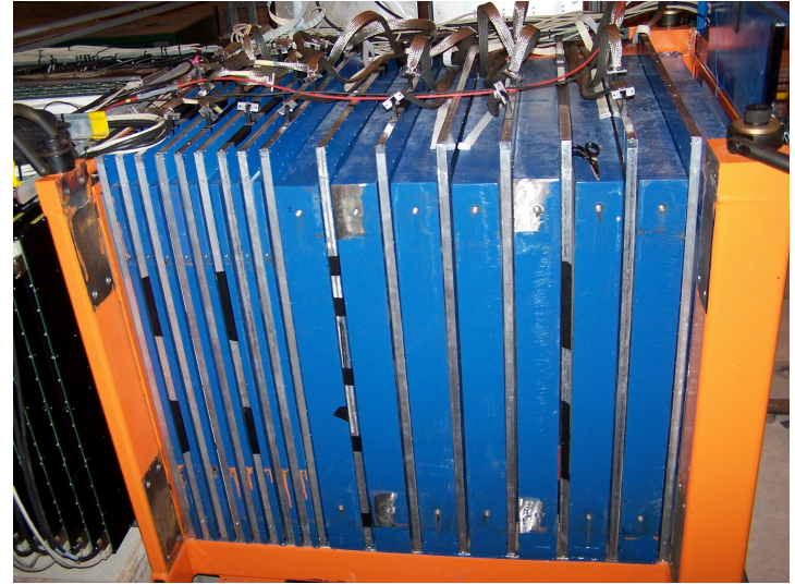
TailCatcher and MuonTracker is an iron-scintillator-sandwich-calorimeter using SiPM readout
