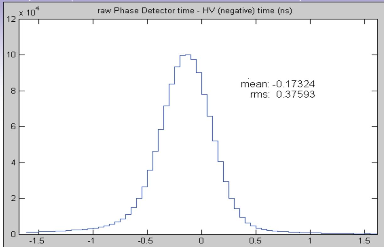
Jitter between raw phase detector signal and FID is  $\sim 375$  ps. If all of this is due to bunch arrival time variations it corresponds to  $\sim 18$  ps jitter in bunch arrival times. (Less if there are other sources of jitter such as the FID trigger circuitry.)
