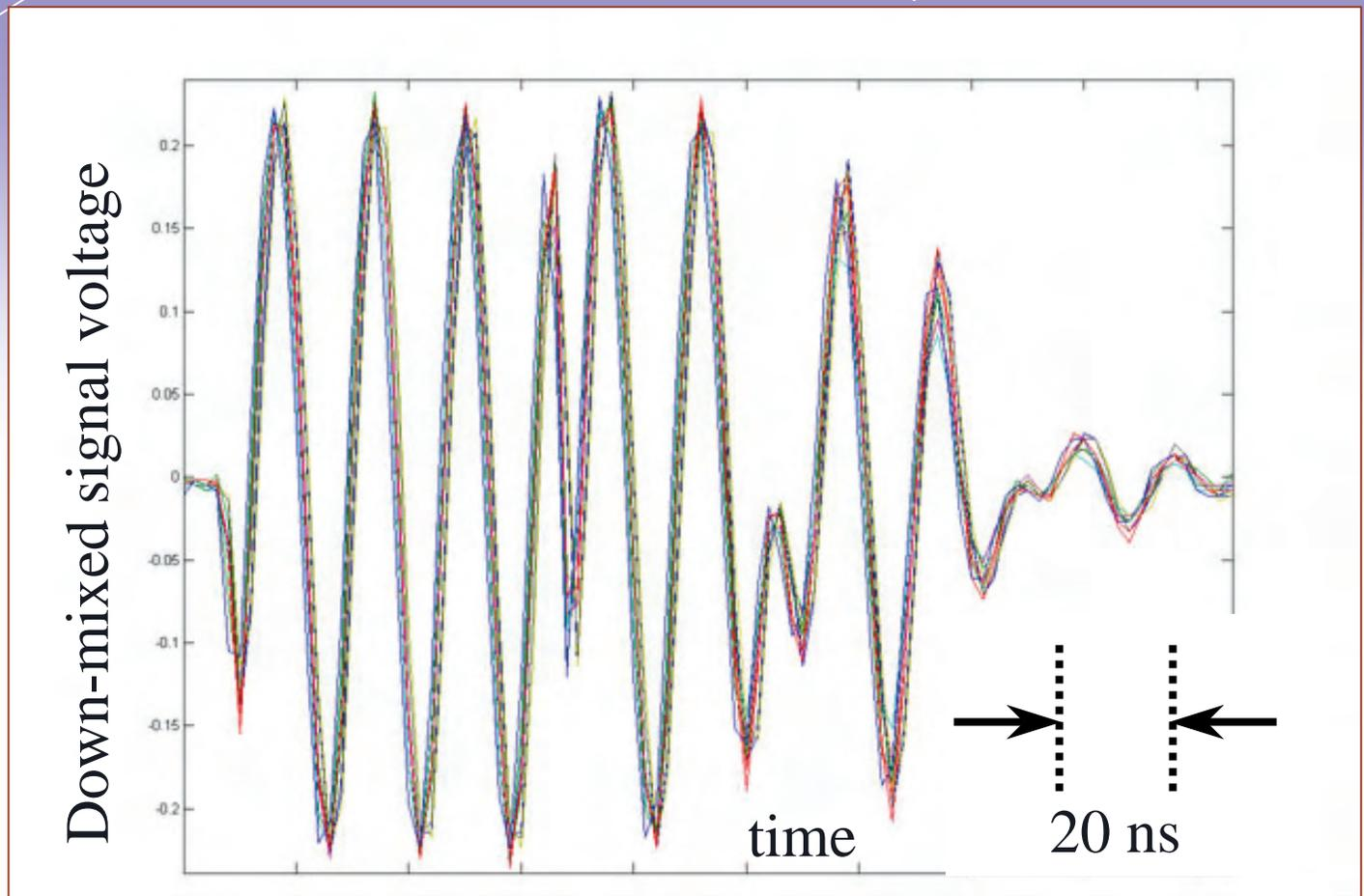
We can probably determine the relative start times for each of the displayed signals with a precision of  $\sim 60$  ps. That maps into a bunch timing measurement accuracy of  $\sim 3$  ps.
