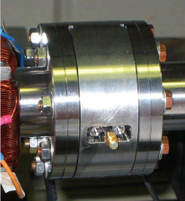
The device produces a very short bipolar signal when a bunch passes through it.
