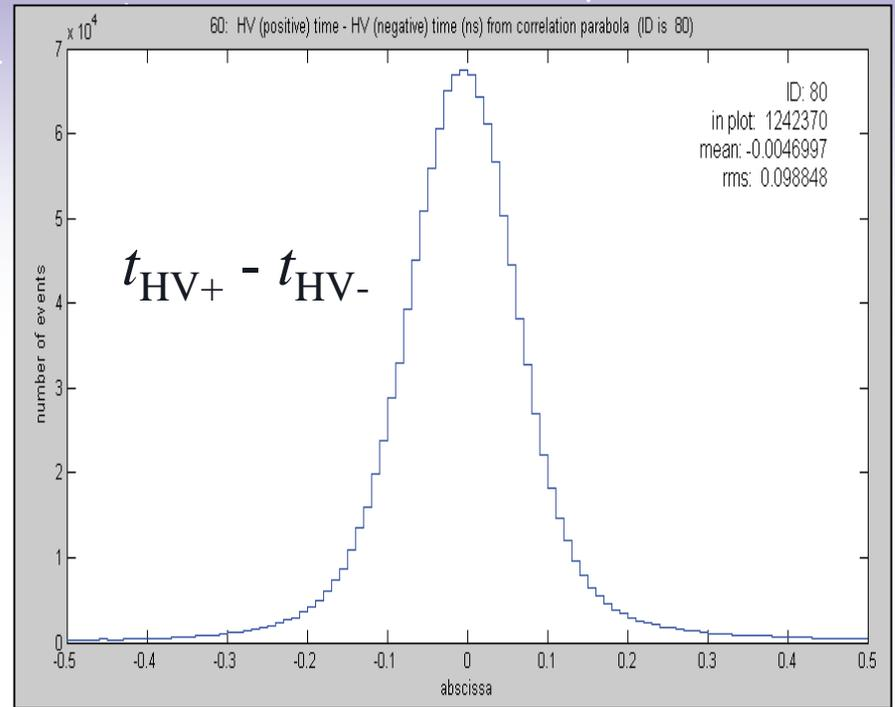
We can determine the relative times of the + and – kicker pulses with a precision of  $\sim 70$  ps if all the jitter is due to resolution. (Even better if some jitter comes from the FID itself.)
