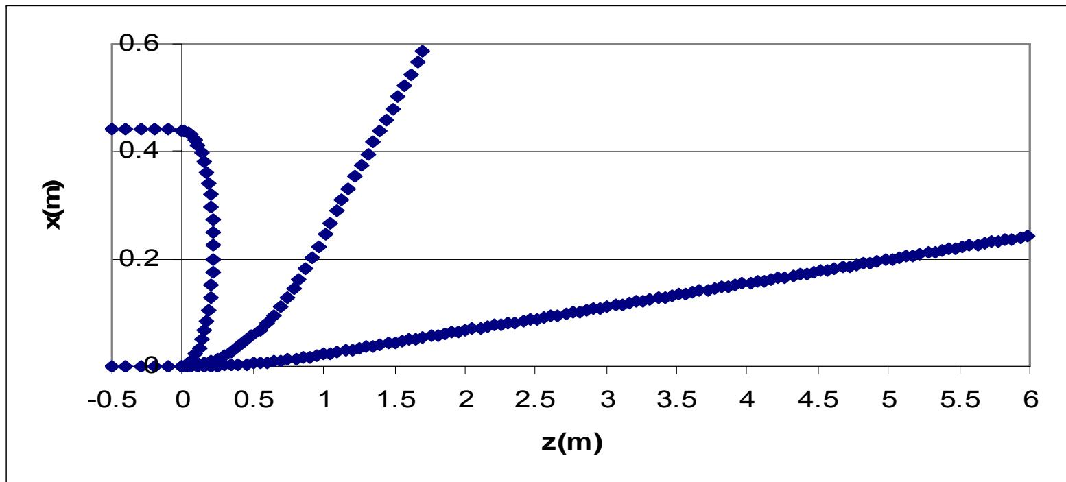
Gas jet followed by a 1m long 1.5T dipole magnetic field. Trajectories of positrons of momentum 0.1, 1, and 10 GeV/c are shown.
