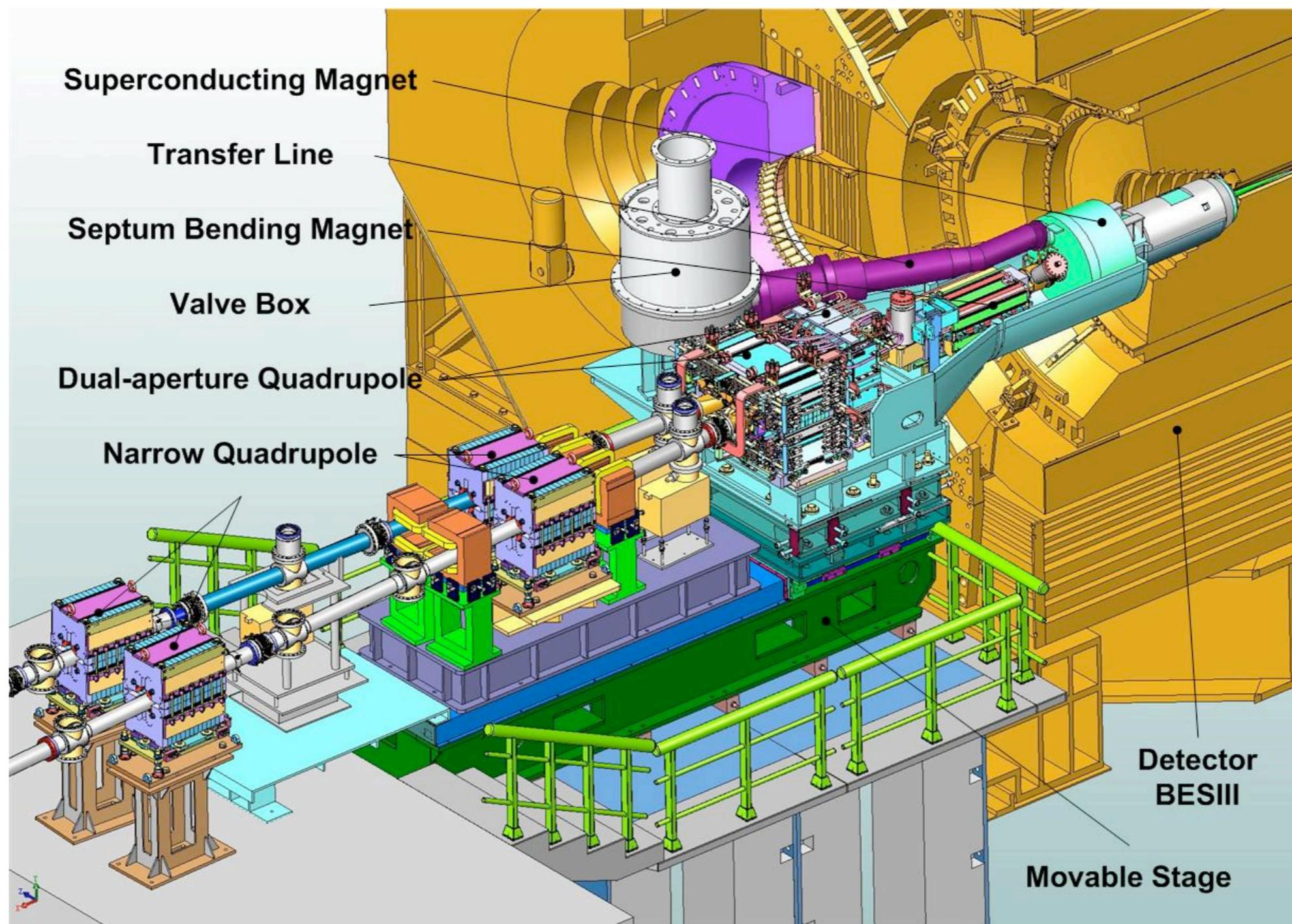
**Vacuum chamber will be finished in Apr. The test of superconducting magnets will begin in Jul. Integration and commissioning of BEPCII IR are planned at the end of this year.**
