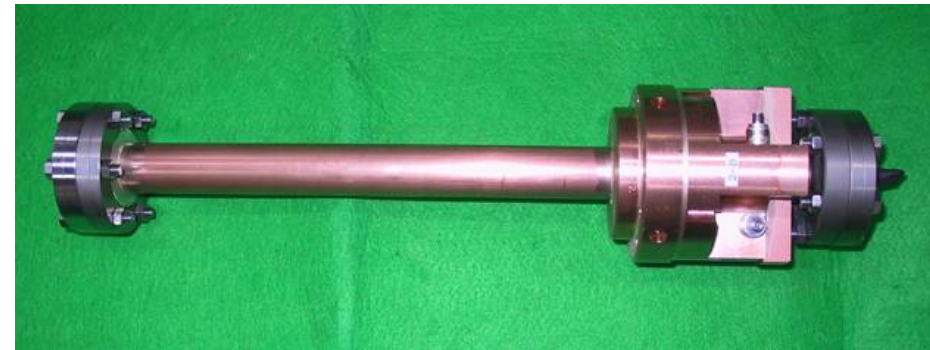
Photo of Production Cavity BPM with Beam Pipe
