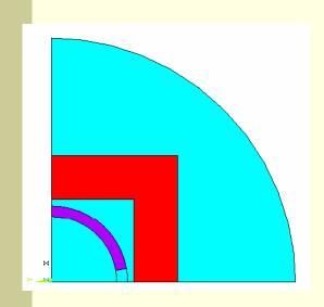
Geometry of the flux return: naïve attempt to force the flux lines to bend more
