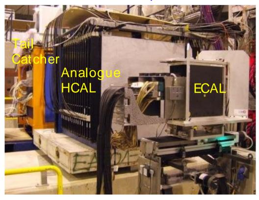
O(15000) calorimeter cells readout by Calice DAQ
