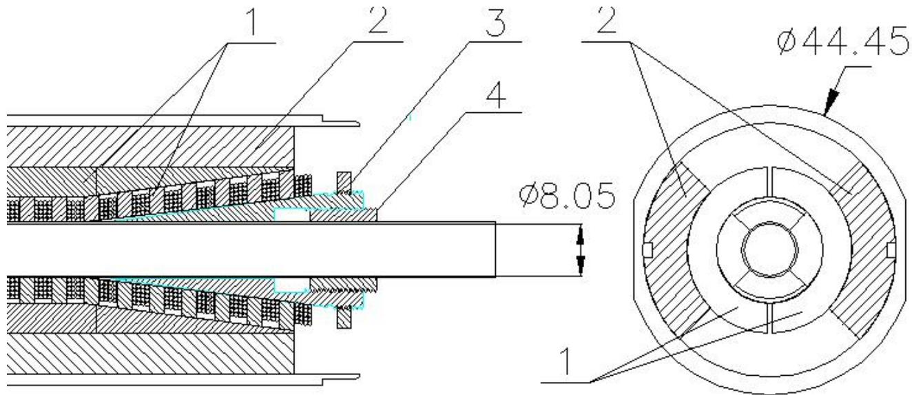
Details of design. 1–Iron yoke, 2–Copper collar, 3, 4–trimming Iron nuts. Inner diameter of **Copper** vacuum chamber is 8mm clear.
