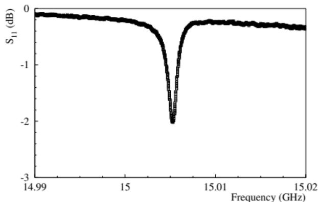
$Q_U$  is larger than expected, because a fraction of the scattered power does not leave the resonator and oscillates between the mirrors (not considered in the theoretical estimation of  $Q_S$ ). If the mirrors are further apart, this effect becomes smaller: the expected and measured  $Q_U$ -values agree.
