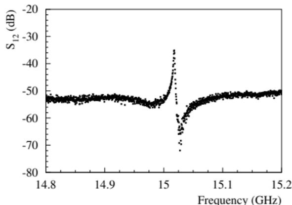
$S_{11}$  measurements suggest that the iris scatters power out of the resonator. By reciprocity, external fields may couple to the iris: around 15 GHz, a fraction of the radiated power is trapped in the resonator and transmitted into the waveguide, leading to the observed pattern for  $S_{12}$ .
