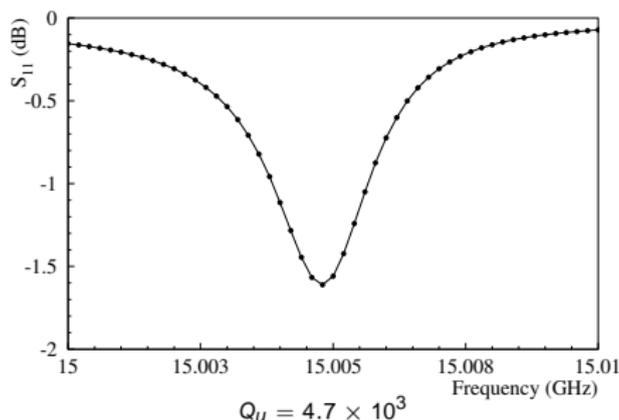
One should not take for granted the quality factor derived with FEMLAB. For instance, it is very sensitive to the mesh. Also, the low-reflecting boundaries used in FEMLAB do not strictly behave as open boundaries.
