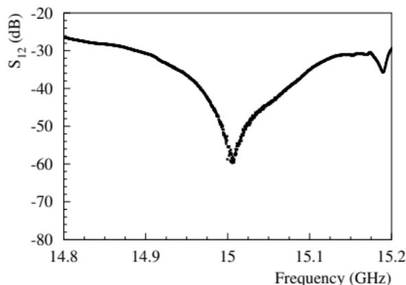
The rejection of parasitic external fields by the nearly confocal resonator prototype is clearly visible.
