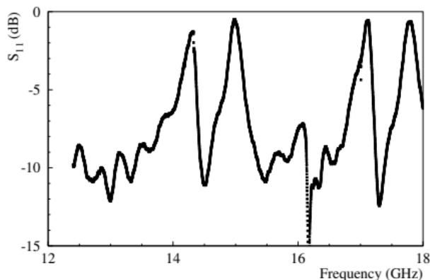
All expected resonances, with small diffraction losses and a non-zero field at the centre of the upper mirror, are observed experimentally.
