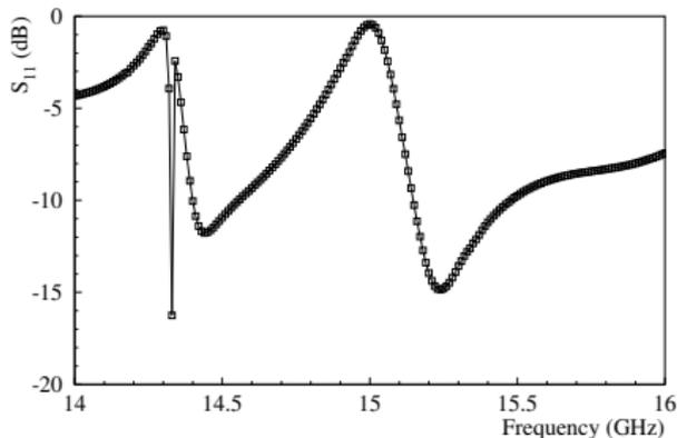
At the resonance, the power injected through the waveguide is trapped inside the nearly confocal resonator, which has small diffraction losses. So, most of the power oscillating between the mirrors couples back to the waveguide, and  $S_{11}$  is close to 0 dB.
