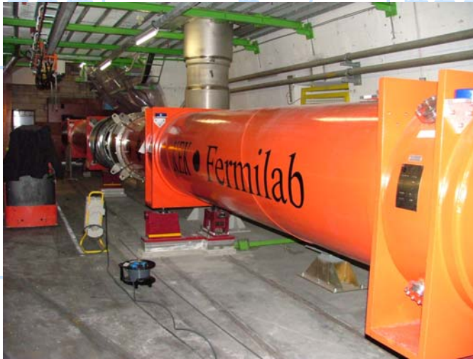
LHC low beta quadrupole next to ALICE Interaction region
