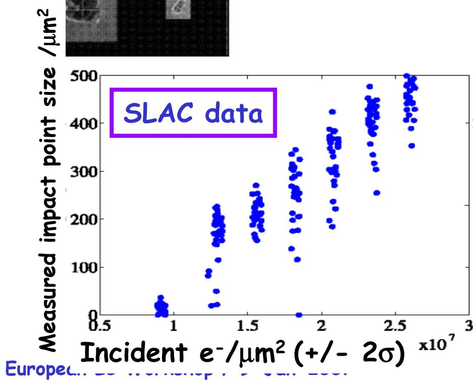
Fluka prediction of beam damage, good agreement with data (NB: evaporated vs. melted - expect data < FLUKA)
