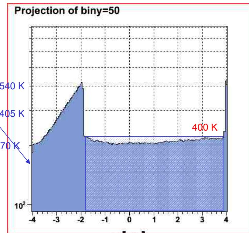
$\Delta T_{\text{max}} = 580$  K per a bunch of 2E10 e- at 500 GeV
