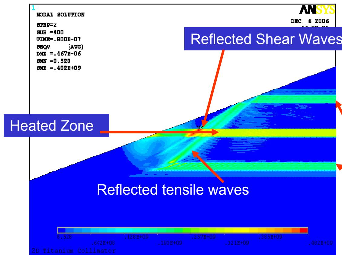
Most damage caused by reflected shear waves
