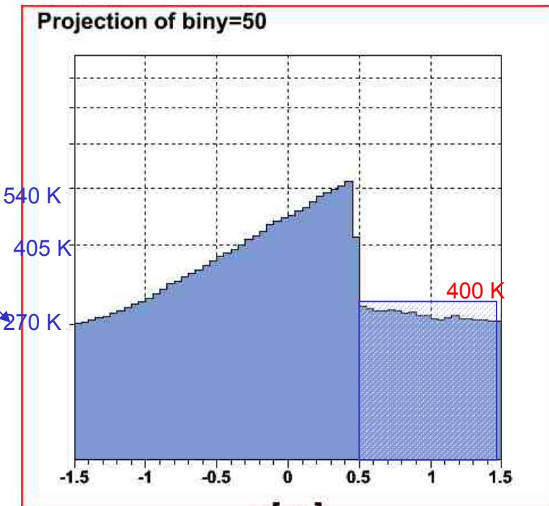
$\Delta T_{\text{max}} = 575 \text{ K}$  per a bunch of  $2E10$  e- at 500 GeV
