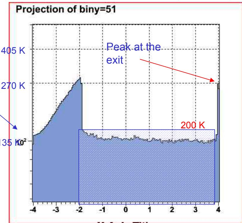
$\Delta T_{\text{max}} = 295$  K per a bunch of  $2E10$  e- at 250 GeV
