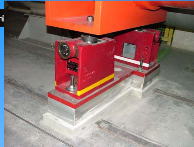
View of the alignment jacks. Note the enlarged contact section and the extra layer of concrete.
