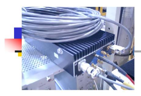
BPM electronics for cavity-BPM (SLAC)
