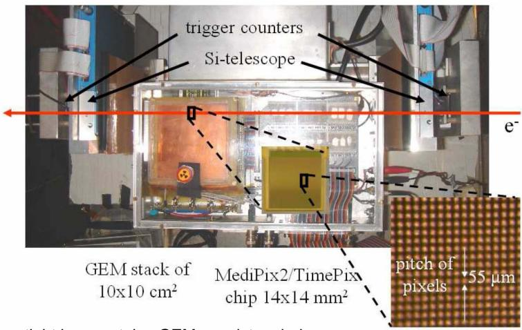
• Gas tight box contains GEMs, resistor chain, TimePix and MediPix2 chip and readout electronics of pads
