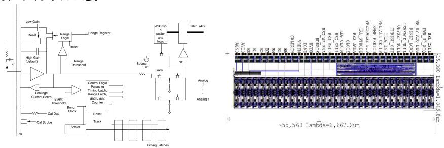
Several KPiX versions made, tested - about to be applied to GEM-DHCAL; integration with ECAL sensor soon.
