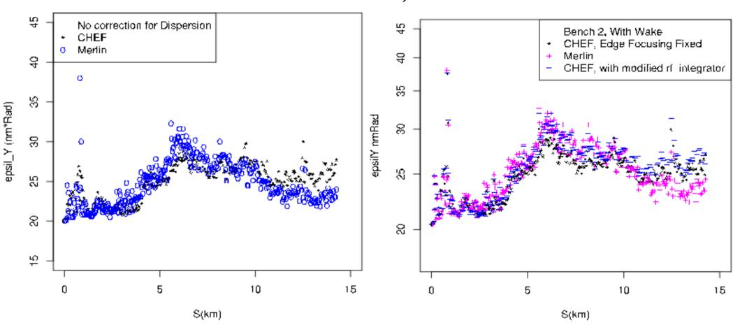
Discrepancy in the emittance spike, at z = 0.8 km, understood and "fixed" "Systematic error" of  $\sim 1.5$  nm remains, due to rf Cavity propagator.
