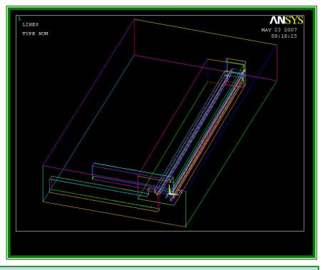
Expanded model to include full conductor and exterior air space surrounding magnet.
