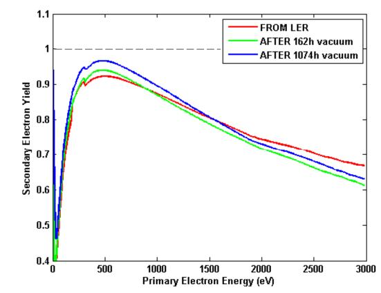
SEY increases slightly if sample is left under vacuum following conditioning in PEP-II LER. Measured SEY after 162h and 1074 hours sitting in SLAC laboratory setup. Average pressure 1.0e-9 torr, 10:1 H2:CO.
