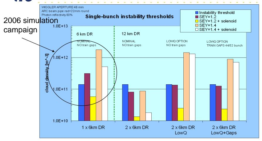
Ring average cloud density. Cloud density (e/m<sup>-3</sup>) <u>near</u> beam (r=1mm) and <u>before</u> bunch passage. Solenoids decrease the cloud density in DRIFT regions, where they are only effective. Compare options 6/12km. All cases wiggler aperture 46mm.
