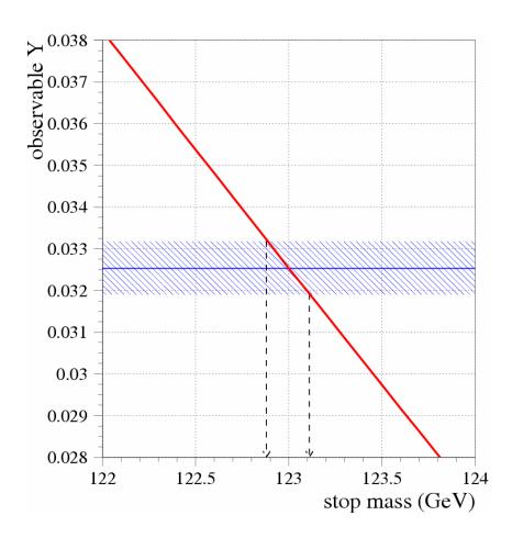
Y=f (M<sub>x</sub>) from the theoretical cross-section is be drawn in Red Y from the data the blue line.
