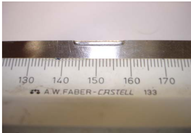
Distortion of the tooling before breakdown
