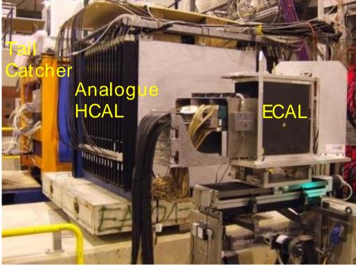
O(15000) calorimeter cells readout by Calice DAQ No Zero Suppression r/o speed 5 Mbyte/s continously
