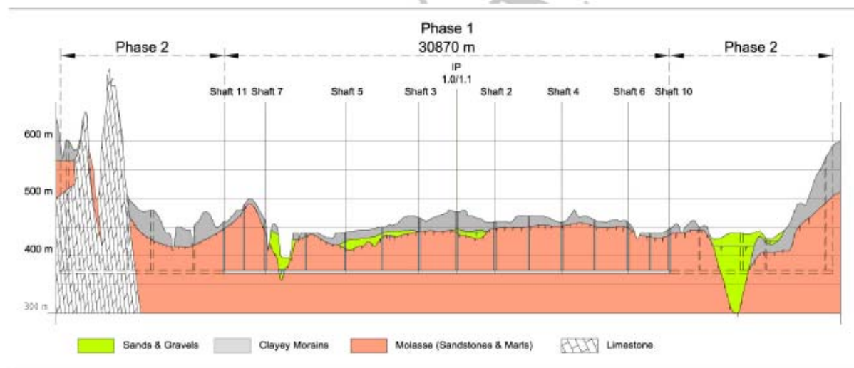
FIGURE 5.4-1. Longitudinal Profile of the European Sample Site near CERN.
