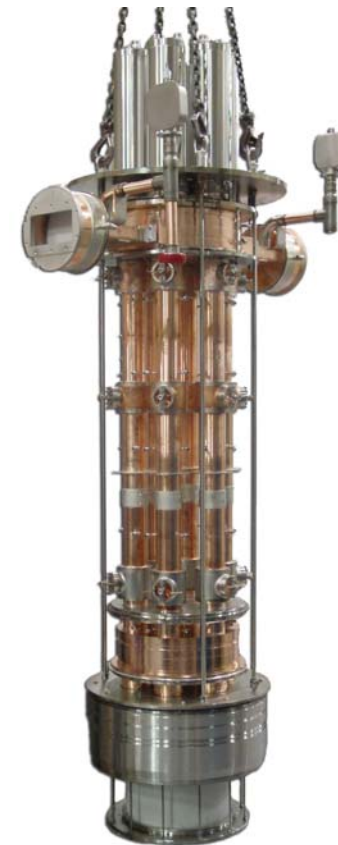
Klystron during construction
