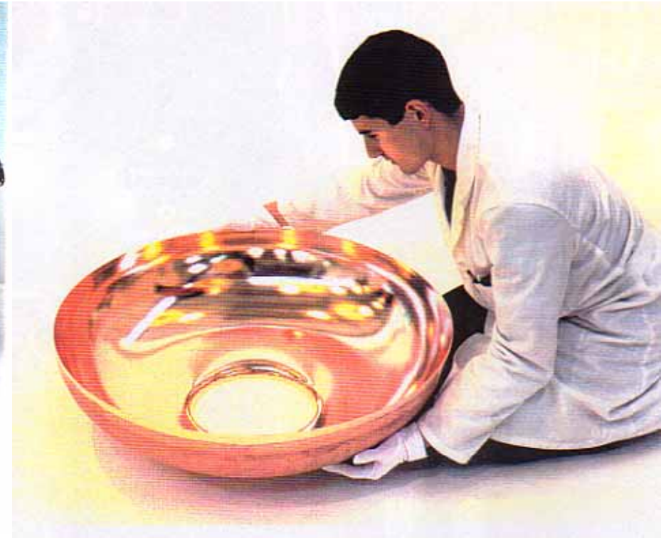
Copper half cell before Nb coating (electropolished)
