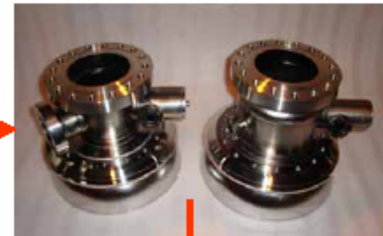
End-beam-pipes with HOM and flanges
