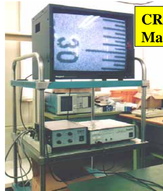
KEK Inner surface inspection system
