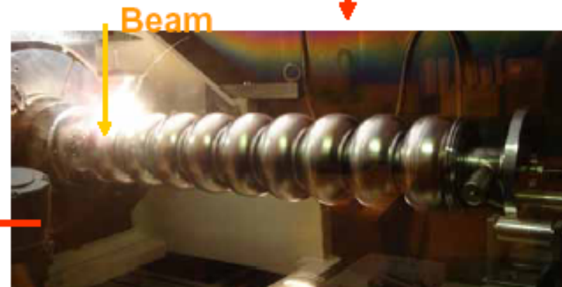
EBW of end-beam-pipes and cell-part
