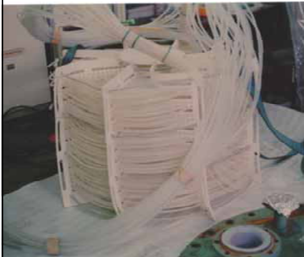
The contaminated heat exchanger
