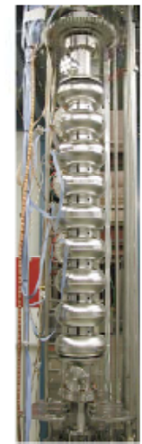
60mm-Aperture Re-Entrant Cavity, 58 MV/m! KEK/Cornell Collaboration
