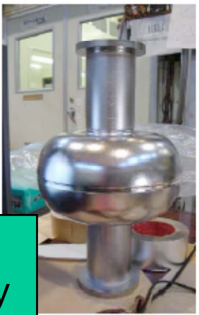
60mm-Aperture Re-Entrant Cavity, 58 MV/m! KEK/Cornell Collaboration
