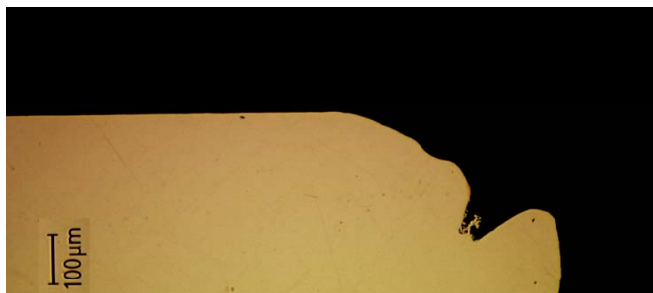
Damaged CLIC structure iris
