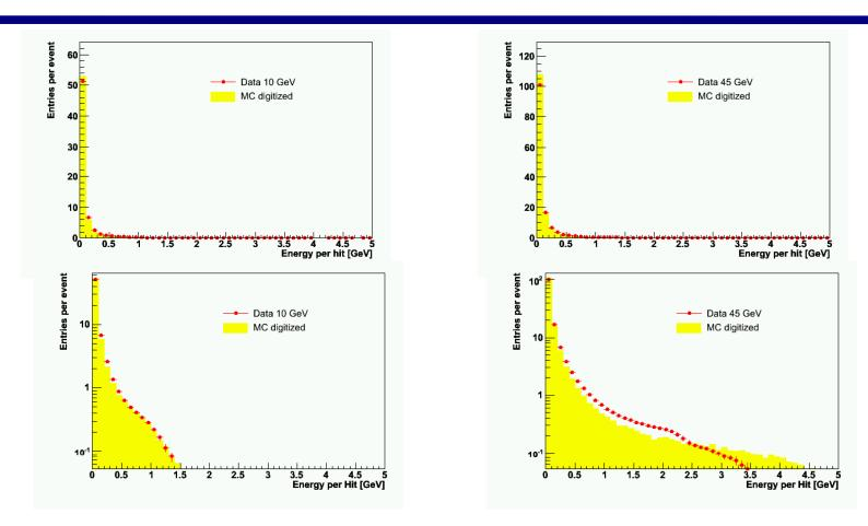
good agreement between data & MC at low energies (<20 GeV) discrepancies at higher energies: beam profile & saturation
