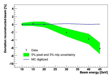
sampling factor  $SF_{data}$  (10~20 GeV): 34.75 MIP/GeV = 0.029 GeV/MIP sampling factor  $SF_{MC}$  (10~20 GeV): 39.99 MIP/GeV = 0.025 GeV/MIP
