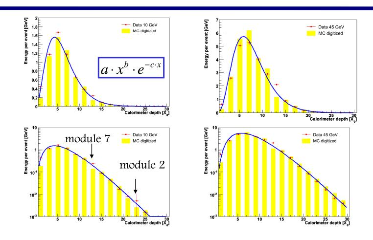
MC shower still starts too late (beam-line material in MC?) module 7: missing ITEP curve for 4 core cells
