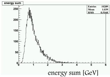
18 noise hits @ 20GeV beam with 1.2 MIP per hit times 1.8\*0.029 GeV/MIP  $\rightarrow 1.1$  GeV noise
