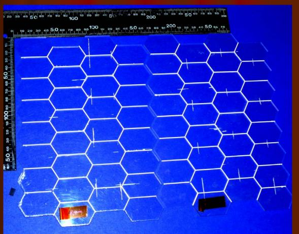
64 small hexagonal cells in one mega cell of EJ-200.
