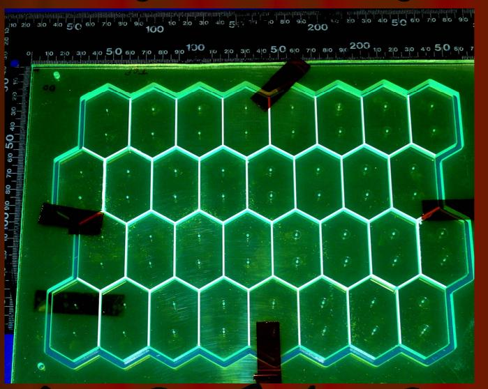
The green emitting plastic scintillator EJ-260 from Eljen Technology with wavelength of max emission at 490 nm
