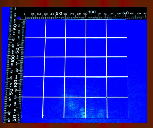
Example of 25 30mm x 30mm square cells of 4mm thickness made of EJ-200 with two aliment holes (next slide)
