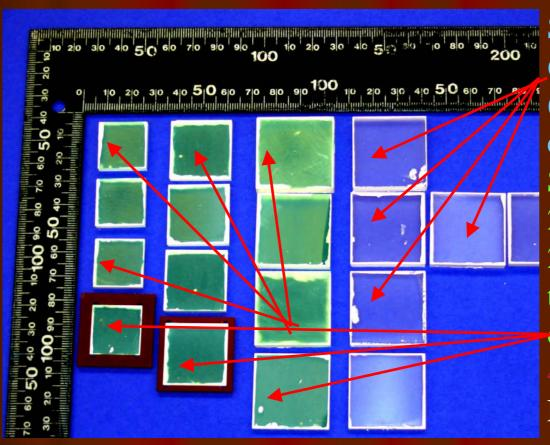
Square 30mm x 30mm EJ-200 6, 5, 4, and 3mm thickness (wavelength of maximum emission is 425nm). Square 30mm x 30mm; 25mm x 25mm; and 20mm x 20mm with 6, 5, 4, and 3mm thickness EJ-260 (wavelength of maximum emission is 490nm).
