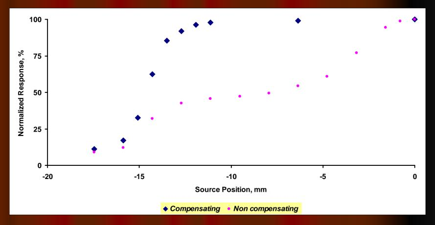
Compensating cells fabricated at NIU were highly uniform.
