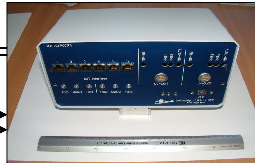
Trigger Logic Unit (TLU) Beam Triggers
