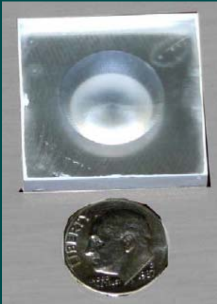
New scintillator design for direct SiPM coupling
