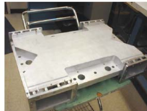
Aluminum Dip-Brazed Prototype
