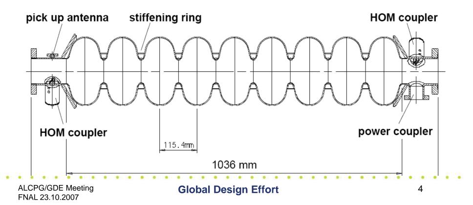
ILC Cavity RF Parameters – Fixed and Changeable
