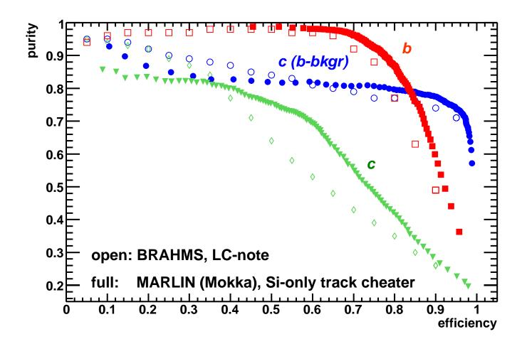
➤ at high efficiency MARLIN(MOKKA) with "Silicon-only" track cheater (VXD, SIT, FTD) gives better performance compared to LC-note result using tracking with pattern recognition
