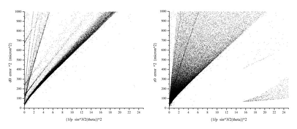
> after correction of the bug by Alexei Raspereza, dependence of track errors in Rφ on momentum and angle looks OK, in z, almost OK, for "Silicon only" tracking
