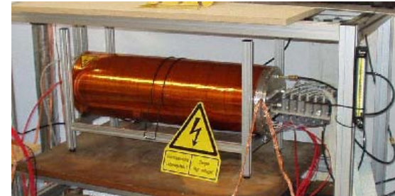
Cornell/Purdue chamber, 64cm drift, 10cm square gas amplification
