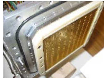
Cornell/Purdue chamber, 64cm drift, 10cm square gas amplification
