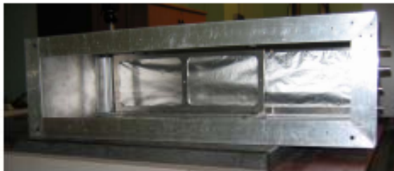
Insulating cage for DESY test beam
