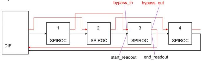
"If e.g. chip 2 fails, chip 1 uses bypass\_out, chip 3 uses bypass\_in".
