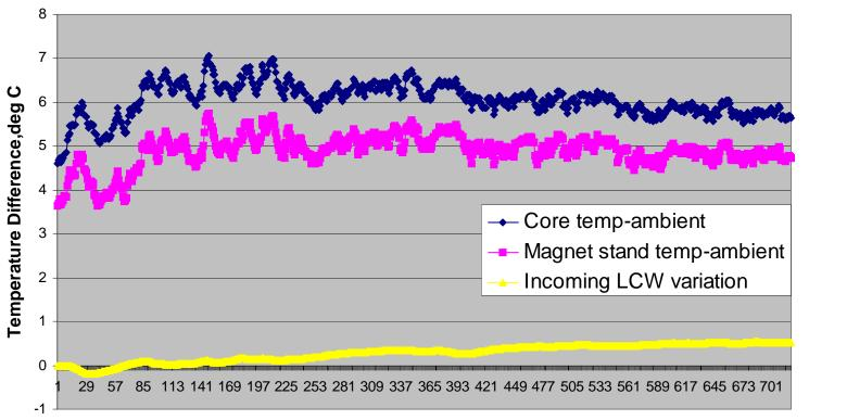
Core & magnet stand temps increase by < 2 C over 4 hour run at 6.5 amps
