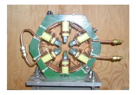
The cooling circuit is one assembly and it all slides into the magnet from one side.
