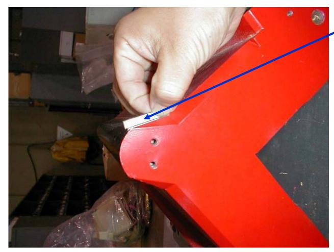
Width of shim carefully chosen so does not interfere with adjacent coil [which vary a little in size from coil to coil] Request to fabricate 16 shims been
