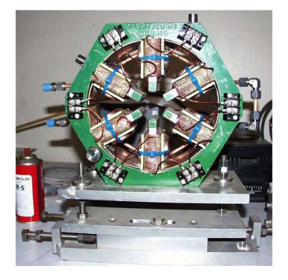
2<sup>nd</sup> version: copper plates on sides of coils, under copper pipes
