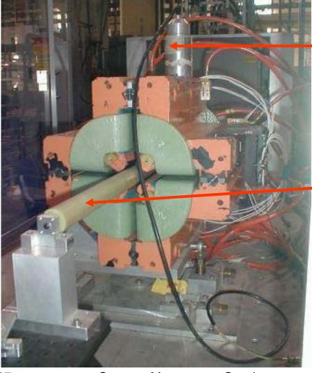
L4 geophone placed for vibration tests (see later)
