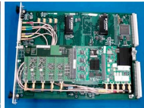
3 rd Generation Field Control Module
