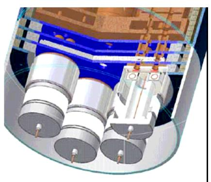
Input and output cavities are common with all beam-lets, While intermediate cavities are independent with one sixth Beams. Six beam-lets has a common filament assembly. Harmonics cavity is introduced.
