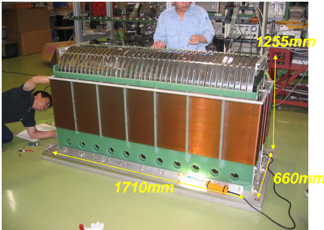
Core-and coil assembly
