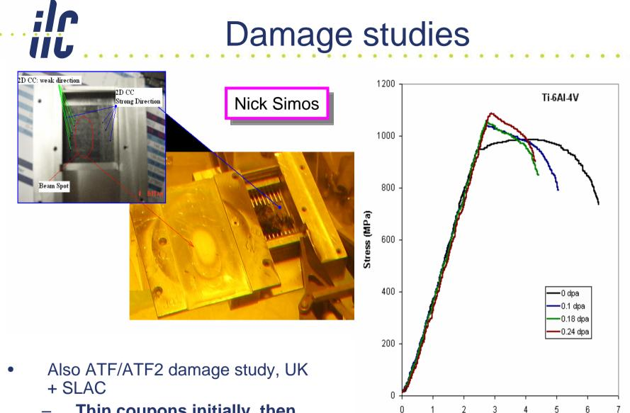
Thin coupons initially, then shockwave measurements by VISAR
