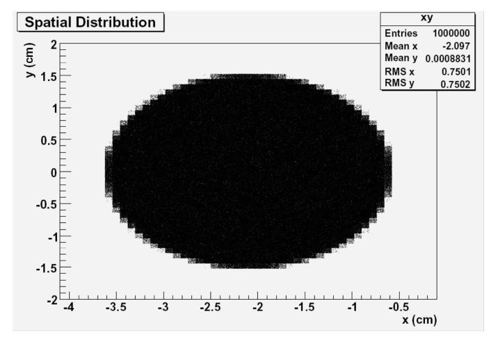
n's randomly and uniformly distributed within the quadrupole bore
