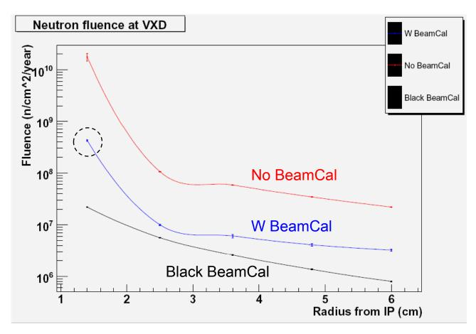
The BeamCal acts as a collimator for neutron backscattering from dump
