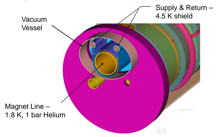
80 K shield is not provided at this cross section A small vent tube for cooldown, not shown, will be added.
