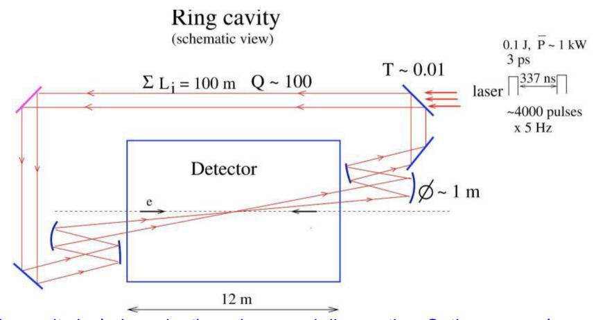
The cavity includes adaptive mirrors and diagnostics. Optimum angular divergence of the laser beam is  $\pm 30$  mrad, A≈9 J (k=1),  $\sigma_t \approx 1.3$  ps,  $\sigma_{x,L} \sim 7$  µm
