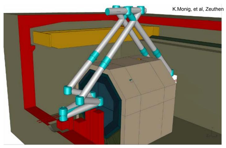
For easier manipulation with bridge crane and smaller vibrations it may be better to hide the laser tubes under the detector. If IR depth is large, the laser room is needed somewhere underground.
