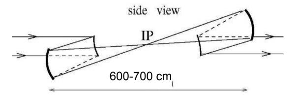
Then the diameter of focusing mirror is about 20 cm and that of the auxiliary mirror about 11 cm. The dead angle for tracking remains as before about ±95 mrad, but smaller for calorimetry. However, in case mirrors are inside the detector and it is more difficult to adjust optics.
