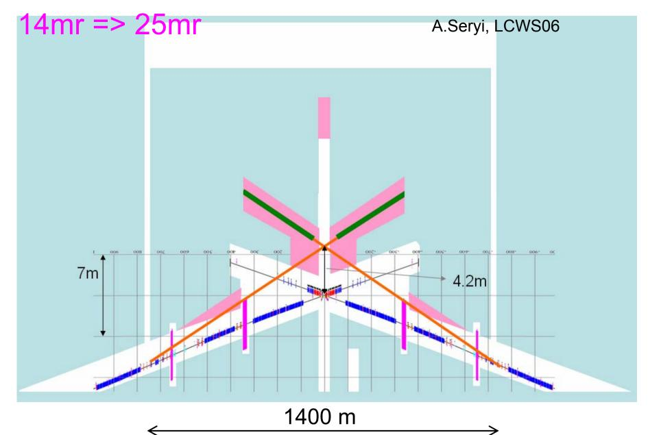
additional angle is 5.5mrad and detector need to move by about 3-4m
