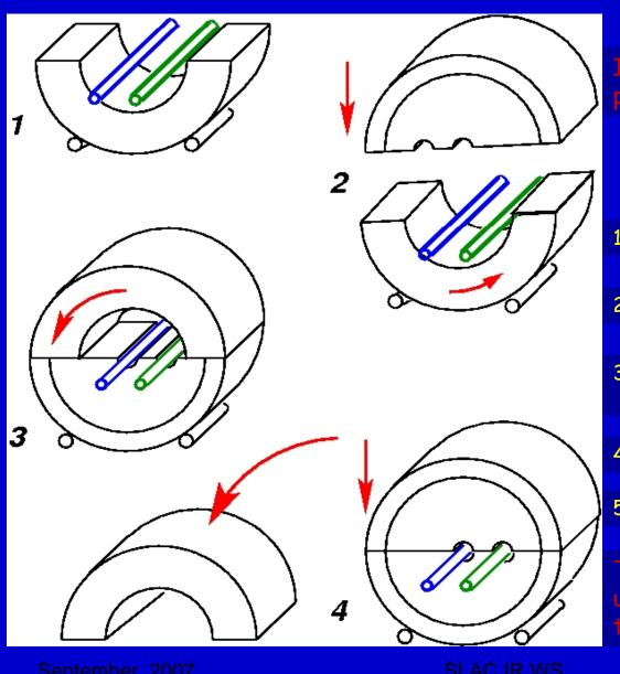
Installation and disassembly must be possible without opening the vacuum!
