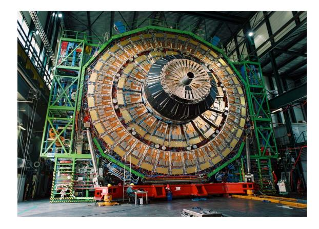
Elements are fully cabled to local racks. All services, gas and water cooling pipes are there. Subdetectors are fully commissioned. Once below they can be connected to the umbilical cables going to the counting rooms through the cable chains.
