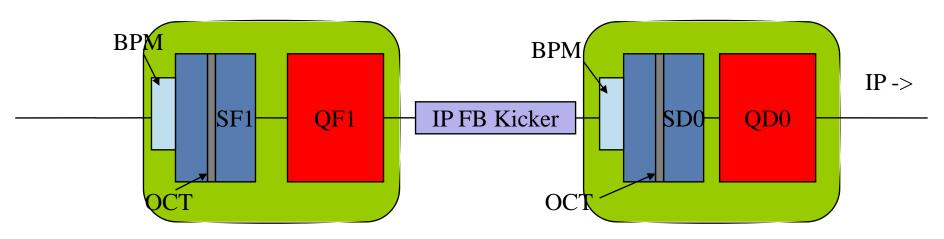
IP FFB kicker (~1m) gap between 2 cryomodules near IP.
