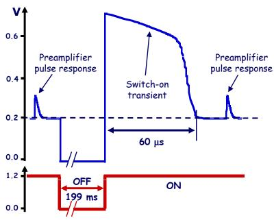
Based on circuit simulations, power cycling with at least 1% duty-cycle seems feasible
