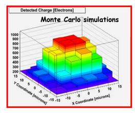
Charge collected by the central pixel in the  $3\times3$  SDRO matrix Physical simulation performed by E. Pozzati - University of Pavia (Italy)
