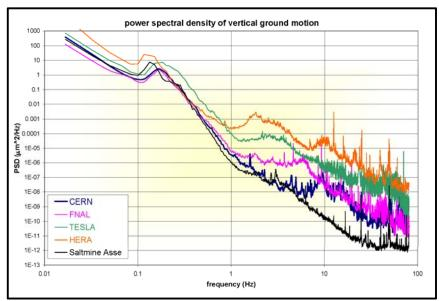
The integrated PSD is related to the RMS  $RMS(f_{1,}f_{2}) = \sqrt{\int_{f_{1}}^{f_{2}} S(f) df}$
