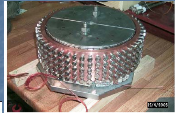
Figure 90 Assembled 1/2 part of superbend pole.
