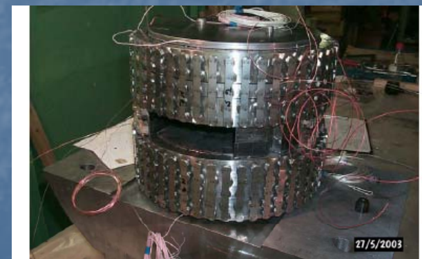
Figure 91 Assembled pole of superbend without yoke.
