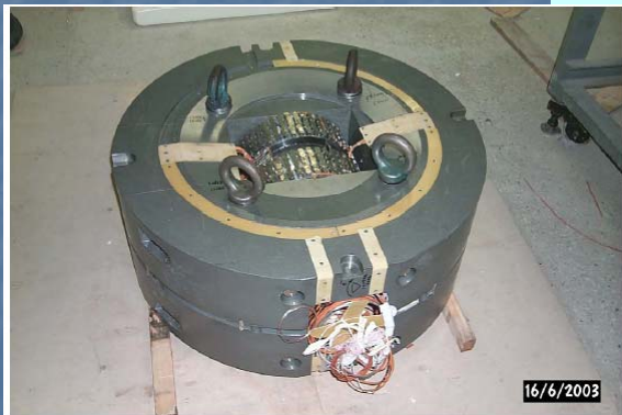
Figure 97 Photograph of assembled superconducting magnet.
