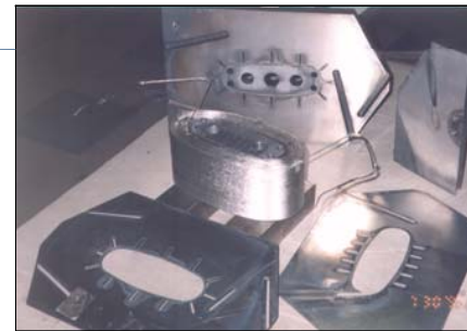
Nb-Sn coil disassembled after baking out
